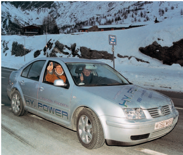
Fig. 4.2-2: PSI tests the experimental car Hy.Power, a modified VW Bora equipped with hydrogen fuel cells and supercapacitors to recover braking energy. The photo shows Hy.Power arriving at the 2005 m high Simplon pass on January 16, 2002 during harsh weather conditions.
